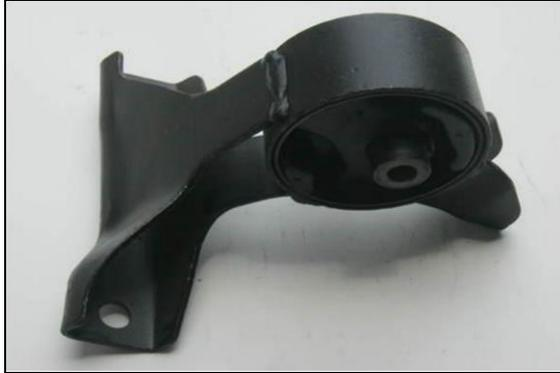
**Fig.1 Potential Application of Composite Material: Engine Mount**      *Investigation*      *of*
