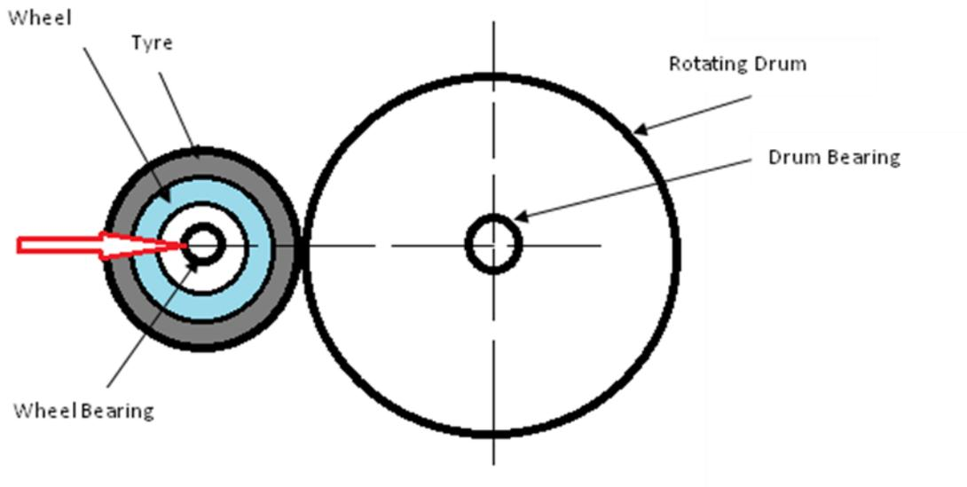
Fig. 1 Schematic test setup of the Dynamic Radial Fatigue Test
