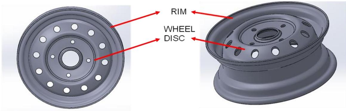
Fig. 2 Solid model of a 12 inch car wheel rim
