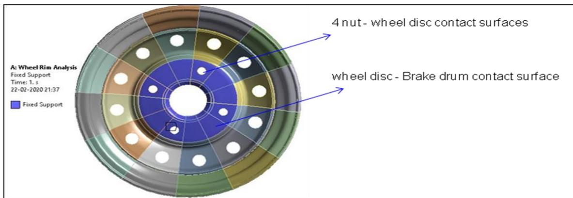
Fig. 7 Fixed Support – 4 nut –wheel disc contact surfaces and wheel disc - Brake drum contact surfaces
