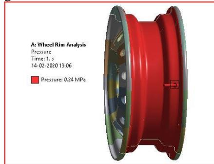
Fig. 8 Pressure applied on outer circumferential surface of rim
