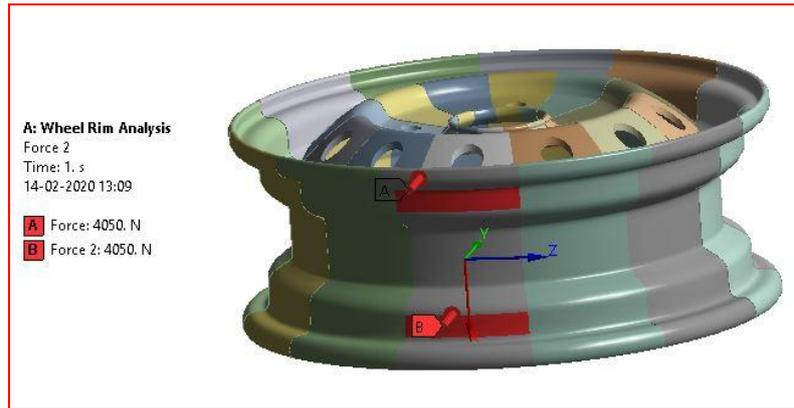
Fig. 10 Radial force F equally distributed as ‘Force’ and ‘Force2’ at two locations
