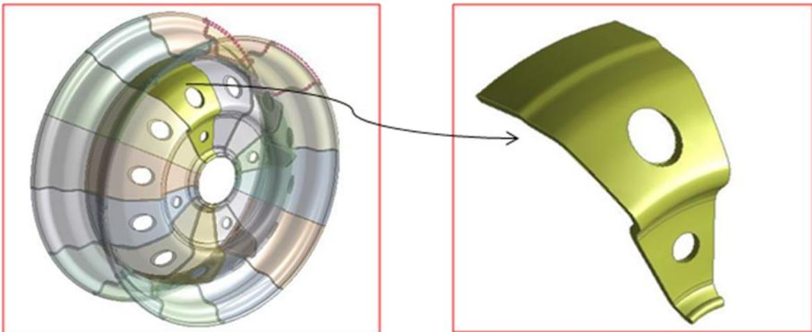
Fig. 5 One of the 12 sectors of Wheel disc
