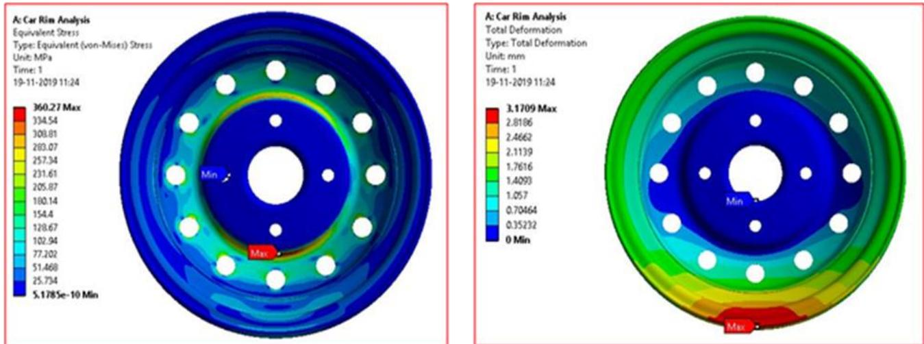
Fig. 12 Von-misses Stress ( MPa ) and Total deformation (mm) for 1.8 mm thick wheel disc in load case-1
