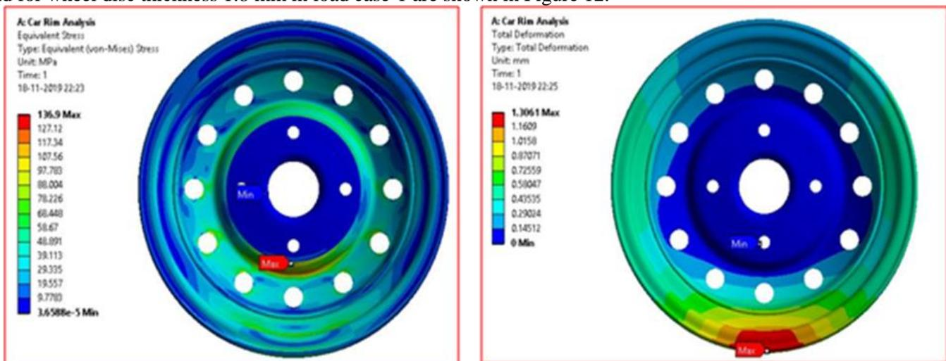
Fig. 11 Von-misses Stress ( MPa ) and Total deformation (mm) for 4 mm thick wheel disc in load case-1
