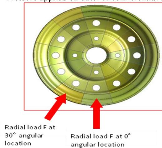
Fig. 9 Angular locations of application of radial load F
