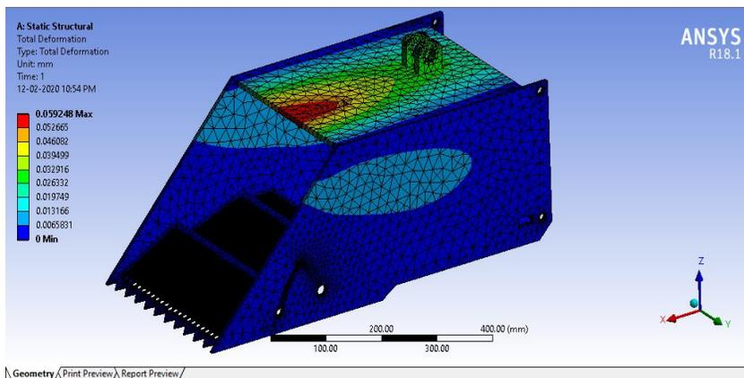
Fig.4 Total deformation for given loading condition
