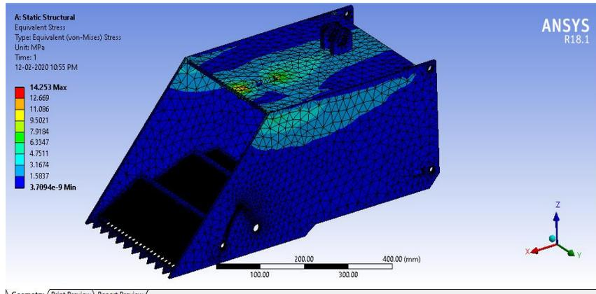
Fig.5 Equivalent stress
