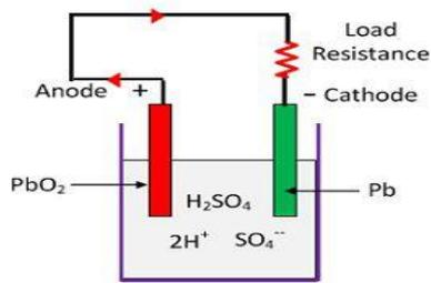
Figure 3: Working of Lead Acid battery.
