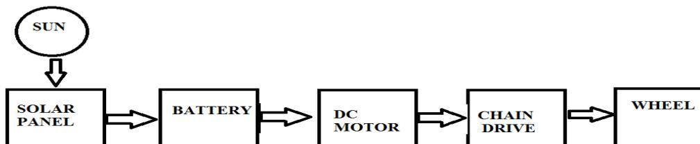
Figure 7: Working mechanism Solar e-bike.
