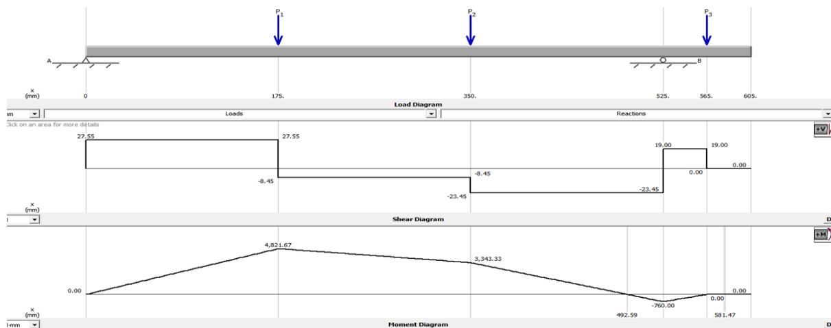
Figure 2: Schematic diagram showing SFD and BMD of vertical loading diagram of input shaft using MD Solid software
