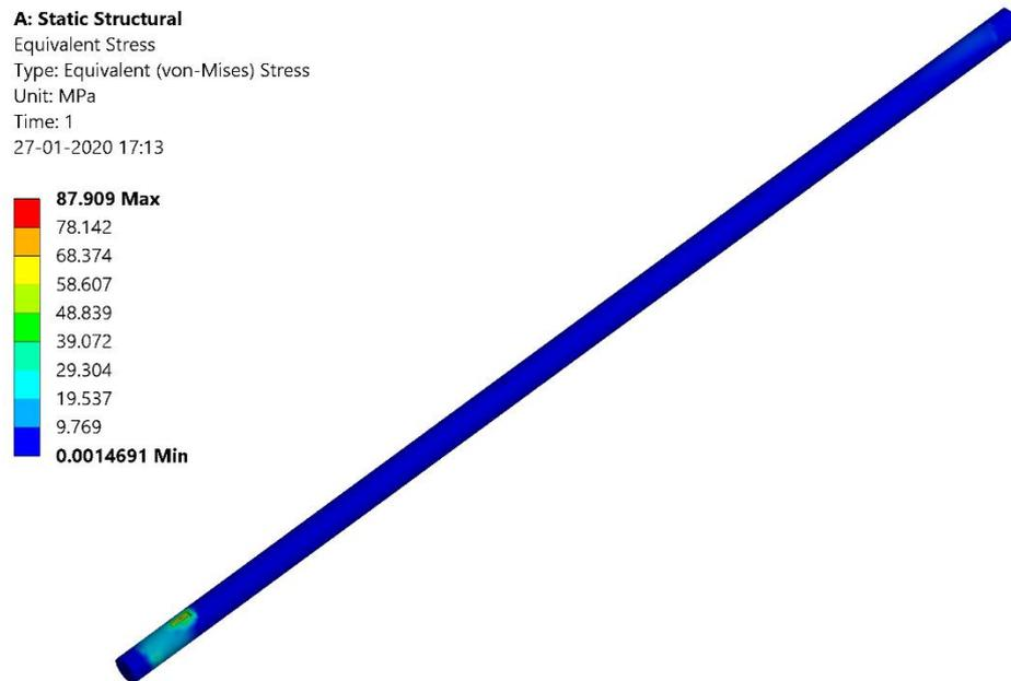
Figure 5: Equivalent Stress distribution on input shaft
