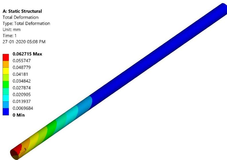
Figure 6: Total deformation of output shaft
