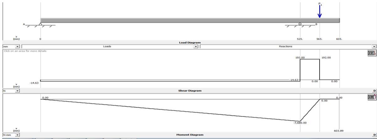
Figure 3: Schematic diagram showing SFD and BMD of horizontal loading diagram of input shaft using MD Solid software
