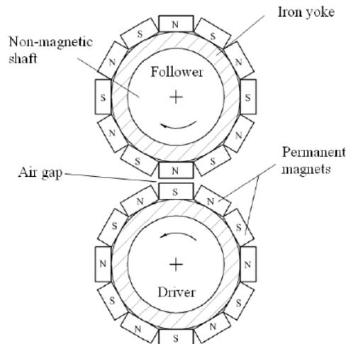
Figure 1: Parallel axis magnetic gears [3]
