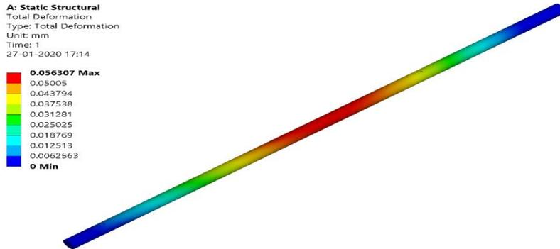
Figure 4: Total Deformation of input shaft
