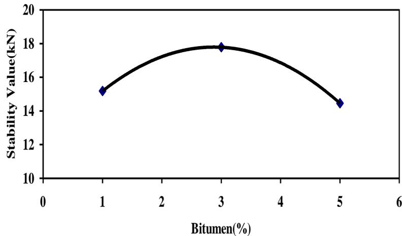
Fig.1 Marshall Stability Curve
