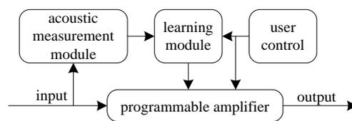
**Figure 3. Structure of User-Programmable Hearing Aids**
