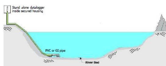
**Figure 5(d). Submersible Pressure Sensor with Standalone Data Logger [16]**
