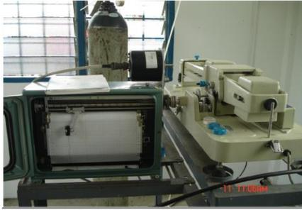
**Figure 6(a). Gas Bubbler System [16]**
