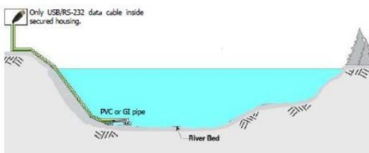
**Figure 5(c). Submersible Pressure Sensor with Onboard Logger [16]**
