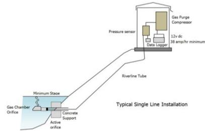
**Figure 6(b). Installation of Gas Bubbler System [16]**
