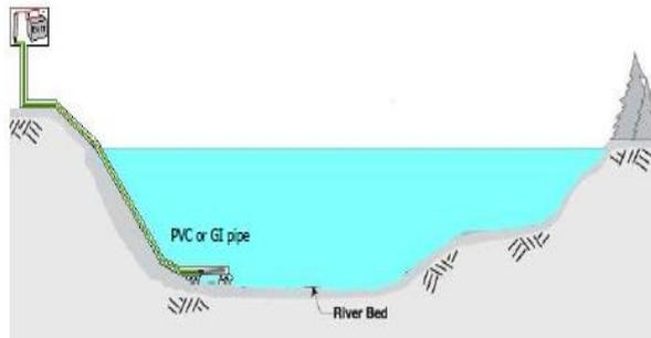
**Figure 5(b). Submersible Pressure Sensor Connected to External Data Logger, Battery and Solar Panel [16]**
