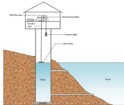
**Figure 4. Drawing of Typical Installation of Digital Shaft Encoder [16]**
