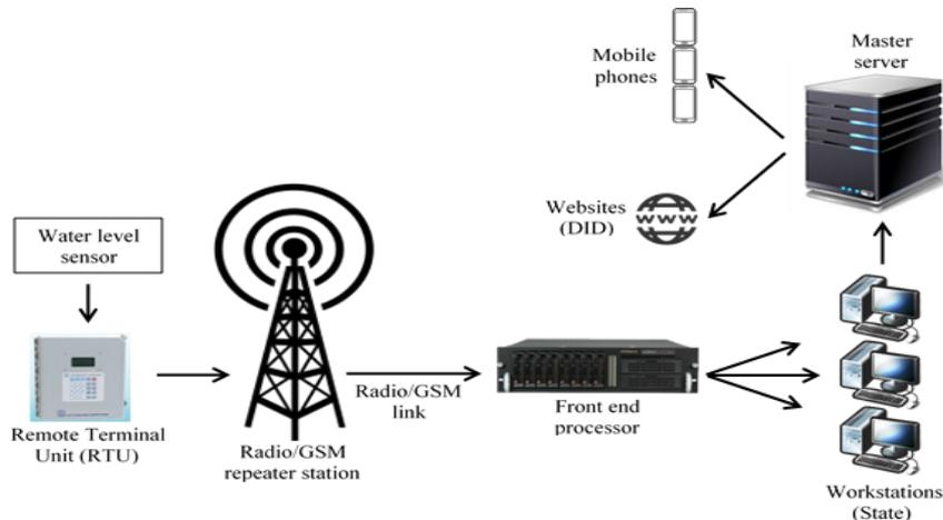
**Figure 8. DID Telemetry System for Water Level Monitoring**
