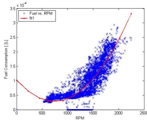
**Fig. 8. Fuel Consumption vs. RPM**
