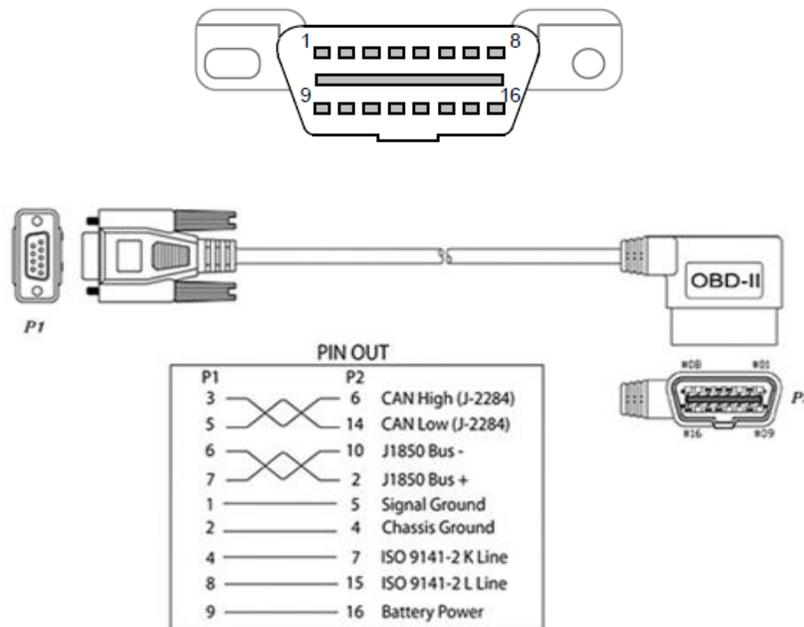
**Fig. 1. OBD-II Port with Pin Layout**
