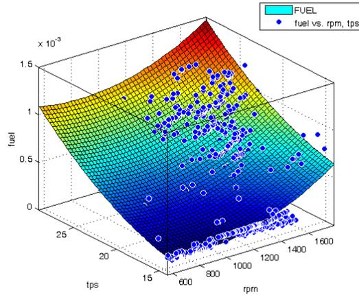
**Fig. 10. Fuel Consumption vs. (RPM, TPS).**
