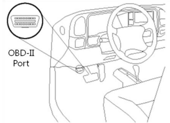
**Fig. 2. OBD-II Port Locates under the Dashboard**
