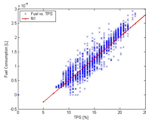
**Fig. 9. Fuel Consumption vs. TPS**
