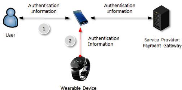
Figure 4. Mobile & Wearable Device-Based 2 Factor Authentication Technique
