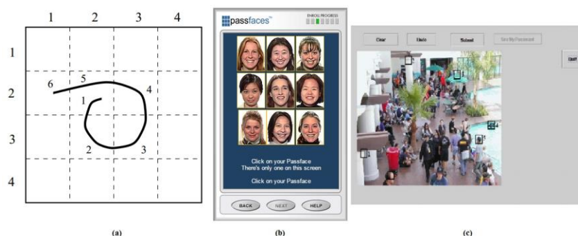
Figure 1. Draw-a-Secret schemata; here a user will draw a figure on an empty canvas, the image is then transformed into a grid resolution and then to a bit representation. This system is aware of changes of the pen stroke, or when the input device is not touching the screen, which is a particular inner
