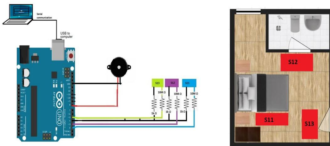
**Figure 2. Circuit Diagram of the Experimental Setup (Left) and 3-D view of the Bedrooms Layout and the Sensor Placement (Right)**
