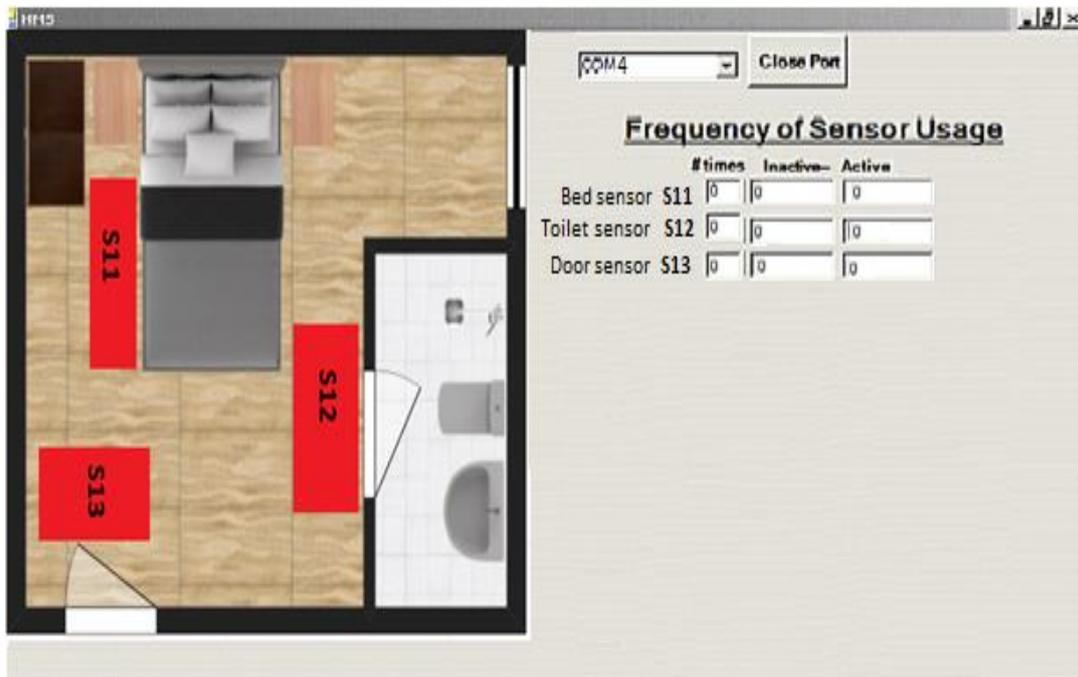
**Figure 3. The GUI Output showing the Active or Inactive Status of the Sensors**
