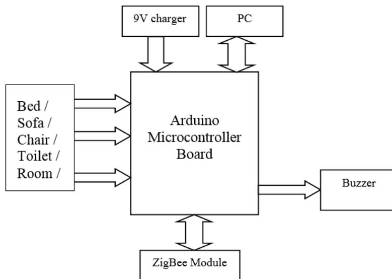
**Figure 1. Block Diagram of the Monitoring System showing the Interfacing Sensors and the ZigBee Module**
