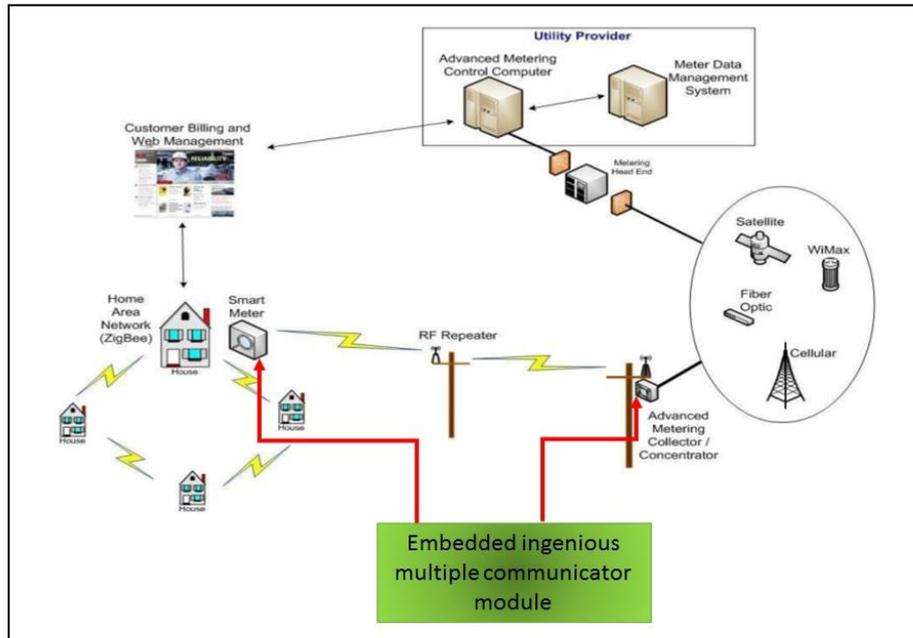
**Figure 6. AMI Topology Reproduced from [17] with Application of Ingenious Multiple Communicator Module**
