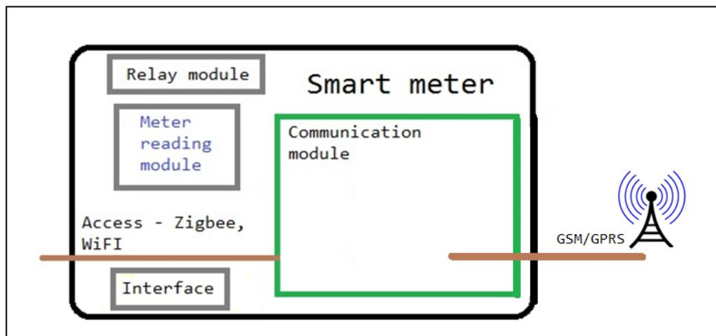
**Figure 2. Single Backhaul Network Connection Smart Meter**
