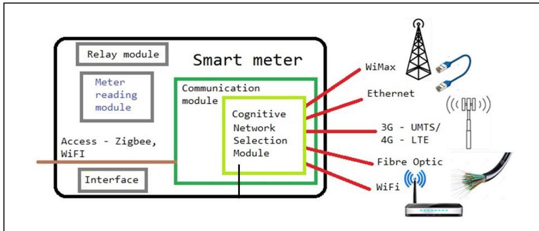
**Figure 3. Proposed Multiple Backhaul Network Connection Smart Meter with Self-Switching Capability**
