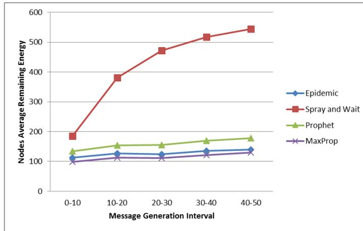
**Figure 5. Nodes Average Remaining Energy vs. Message Generation Interval**
