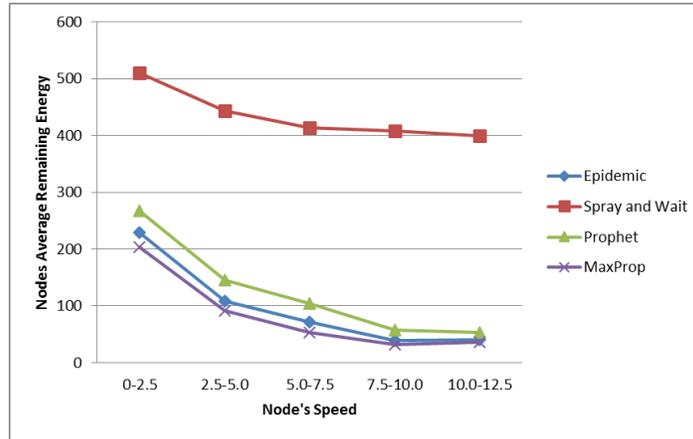
**Figure 7. Nodes Average Remaining Energy as Node speed is Increased**
