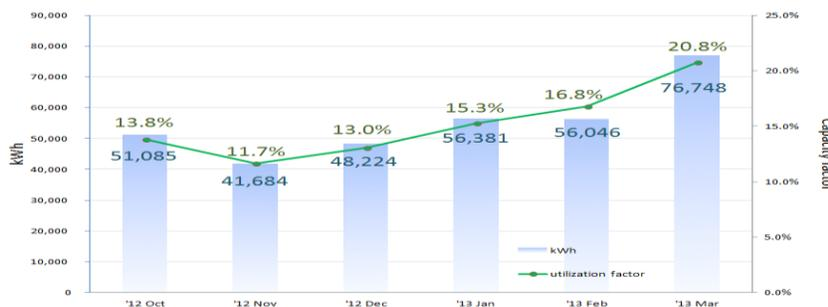
Figure 4. Hapcheon 500kW Floating PV System Performance Analysis Graph
