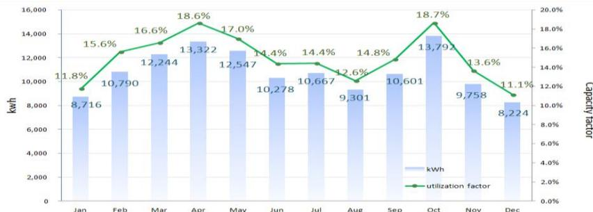
Figure 3. Hapcheon 100kW Floating PV System Performance Analysis Graph
