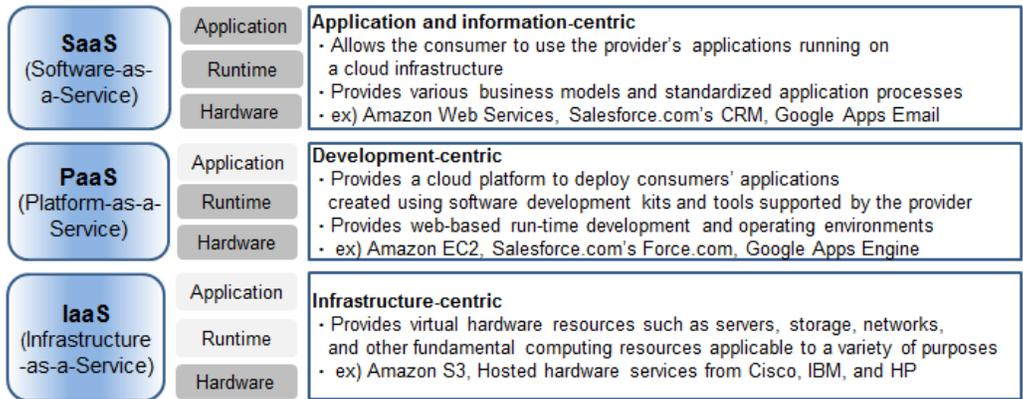
Figure 4. Features of the Three Cloud Service Models
