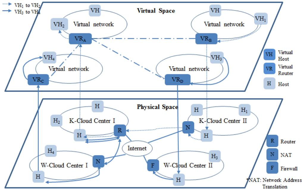
**Figure 8. Configuration of the K- and W-Cloud Centers, Integrated via the ViNe Architecture**
