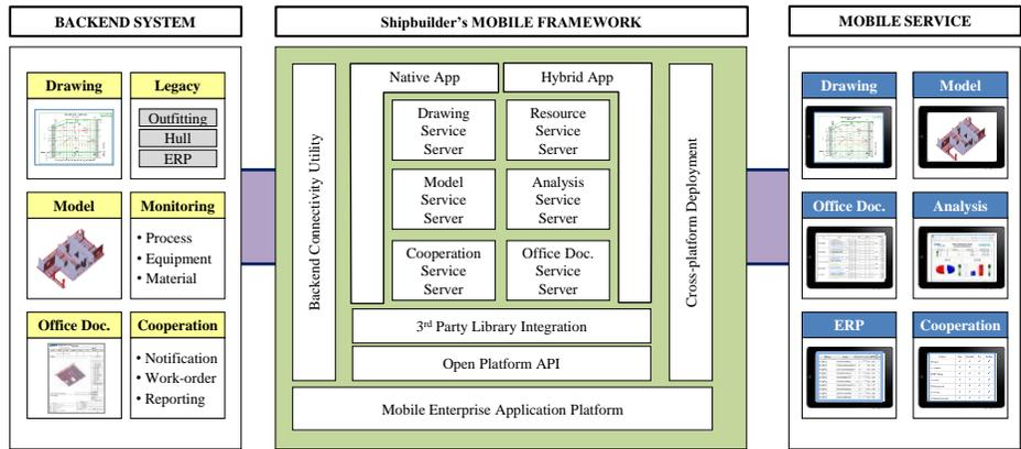
**Figure 1. Shipbuilder's Mobile Framework**
