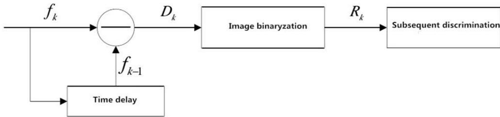
**Figure 2. The Schematic Diagram of the Frame Subtraction Method**
