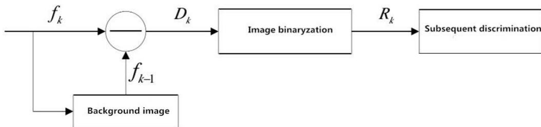
**Figure 3. The Schematic Diagram of the Background Subtraction Method**
