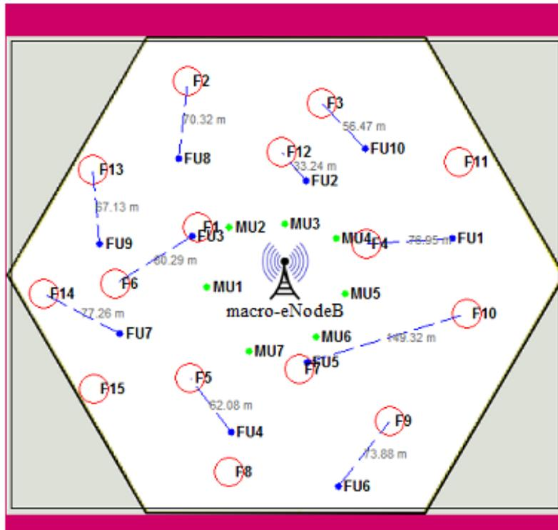
**Figure 3. Simulation Scenario, Where FU Indicates HUE, MU Indicates as MUE, and F States Henodeb**
