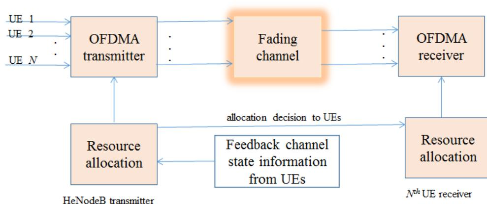
**Figure 2. Multi-User OFDMA System Block Diagram [12]**
