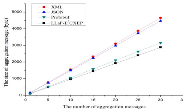
**Figure 2. Length of Different Methods Serialize Aggregation Message**
