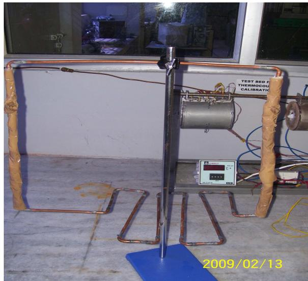
**Figure 1. A Heat Pipe with 5 Turns**
