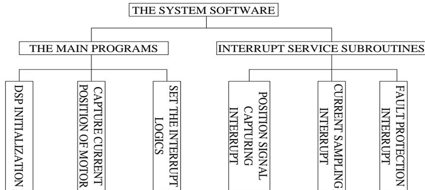
Figure 5. The Block Diagram of the System Software
