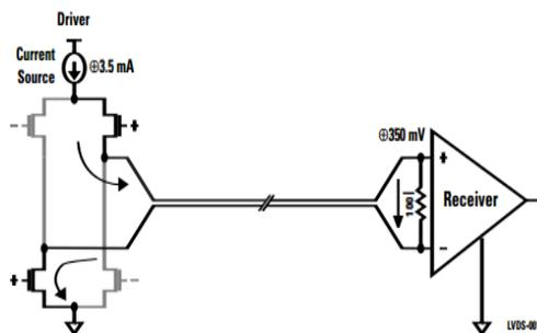
**Figure 1. Diagram of LVDS Driver and Receiver Connected via Differential Impedance Media [7]**
