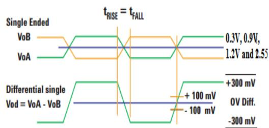
**Figure 2. The Lowered Voltage Swing Maintains High Speed and Consume Less Power [8]**
