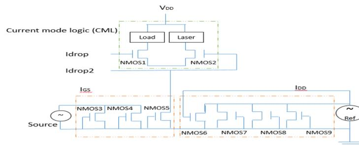
**Figure 5. Laser Driver Circuit using Current Mode Logic**
