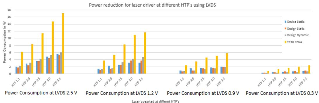
**Figure 7. Laser Driver Power Reduction for different HTP's using LVDS Technique**
