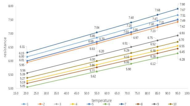
**Figure 5. Resistance Values of PCB Patterns in Table 1 at Each Set Temperature**
