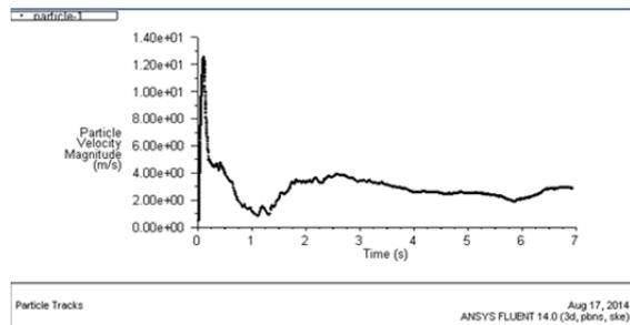
**Figure 12. The Velocity Change Curves of Carrier**
