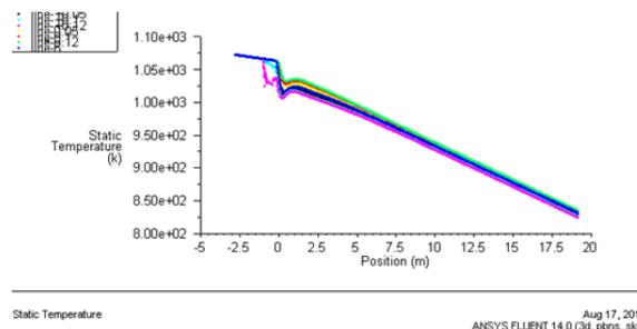
**Figure 6. The Temperature Change Curves of Hot Gas**
