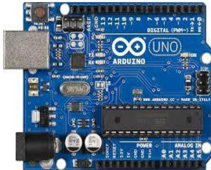
Figure 4. Schematic of Arduino UNO Board [1]
