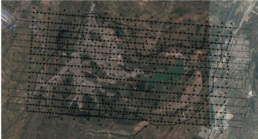
**Figure 1. The Diagram of the Aerial Photographic Route**
