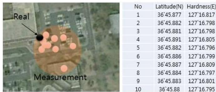
Figure 1. GPS distance errors in a NLOS environment
