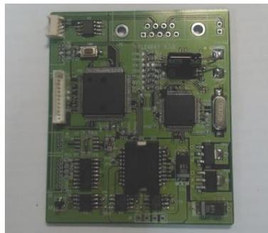
**Figure 6. FlexRay based Motor Control Board**
