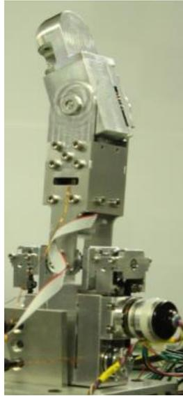
**Figure 1. Structure of the Developed Finger for a Robot Hand**
