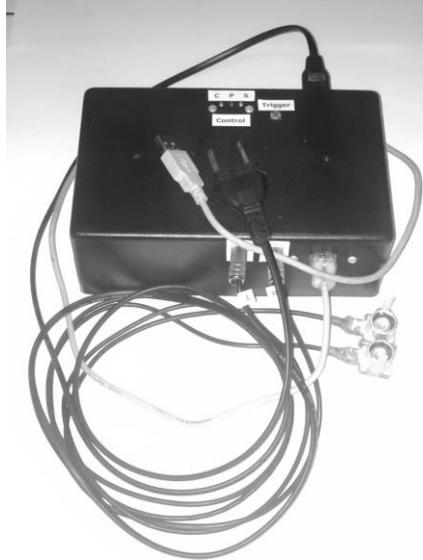
**Figure 4. Ultrasonic signal processing device**
