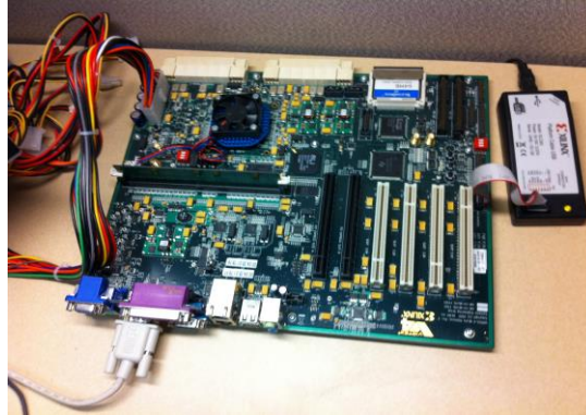
Figure 4. Xilinx ML410 development board to evaluate the proposed adaptive reconfiguration flow for video encoder application
