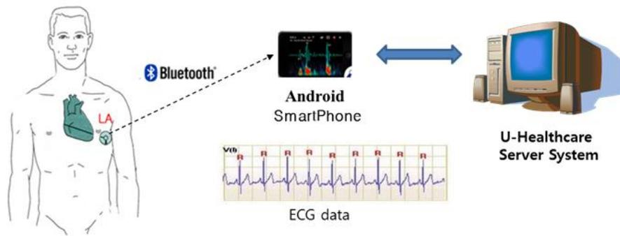
**Figure 1. 5HD Measurement System (ECG case)**
