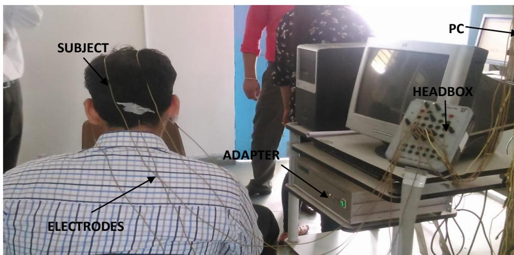
**Figure 6. Experimental Setup for EEG Acquisition**
