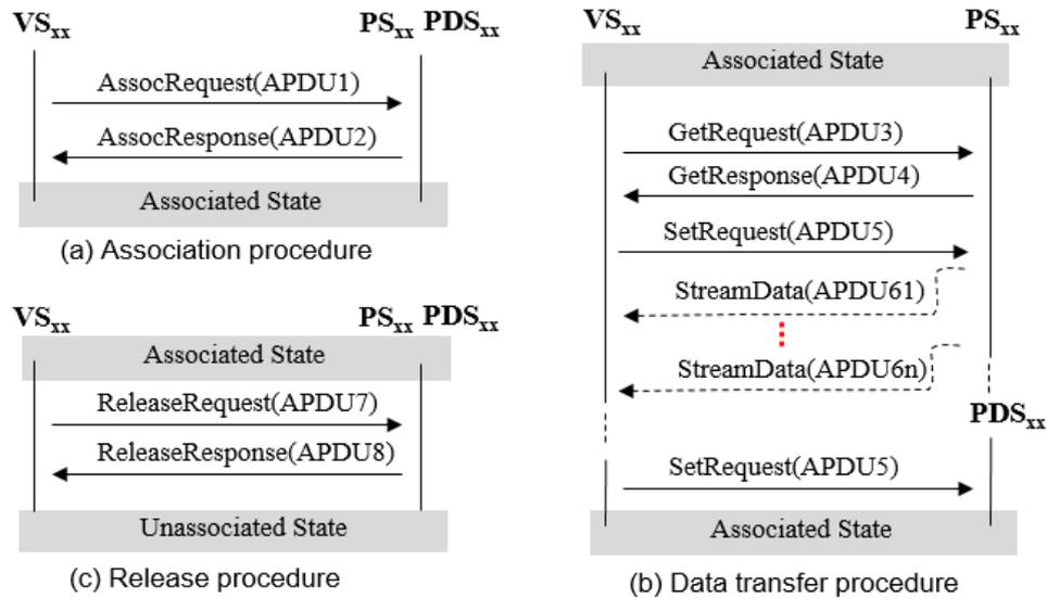
**Figure 3. Application Protocol for Data Transfer**
