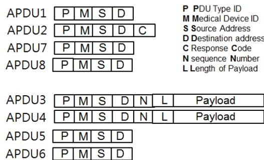
**Figure 4. Application Protocol Data Unit Format**
