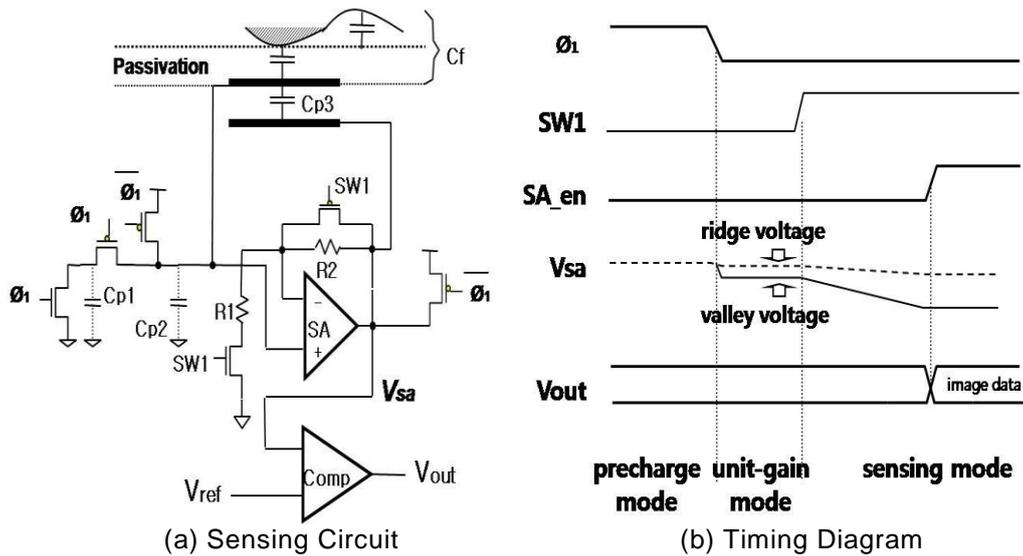
Figure 1. Typical Parasitic Insensitive Capacitive Fingerprint Sensing Scheme
