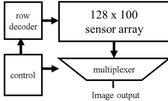
**Figure 8. Chip Architecture**
