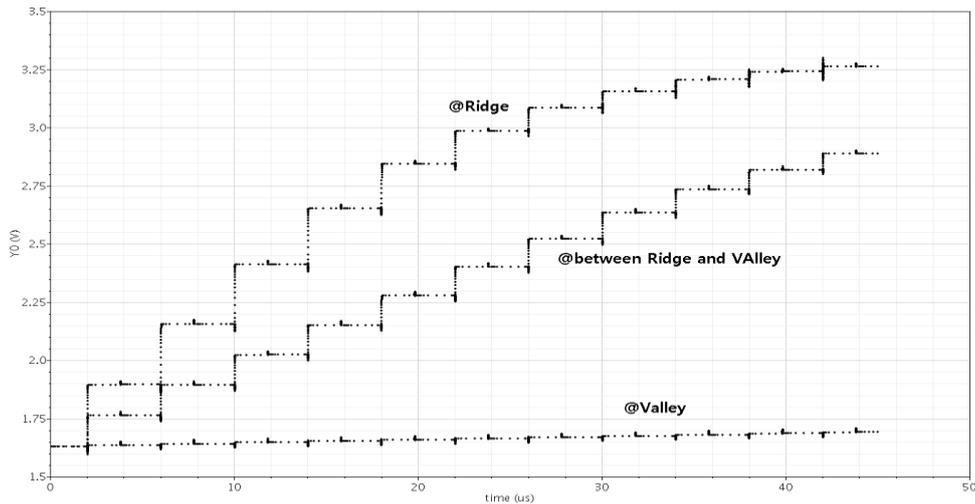
**Figure 6. Time Domain Voltage Output Characteristics of Proposed Sensor Circuit (0.35 $\mu$ m Typical Parameter and 3.3V Power Supply)**
