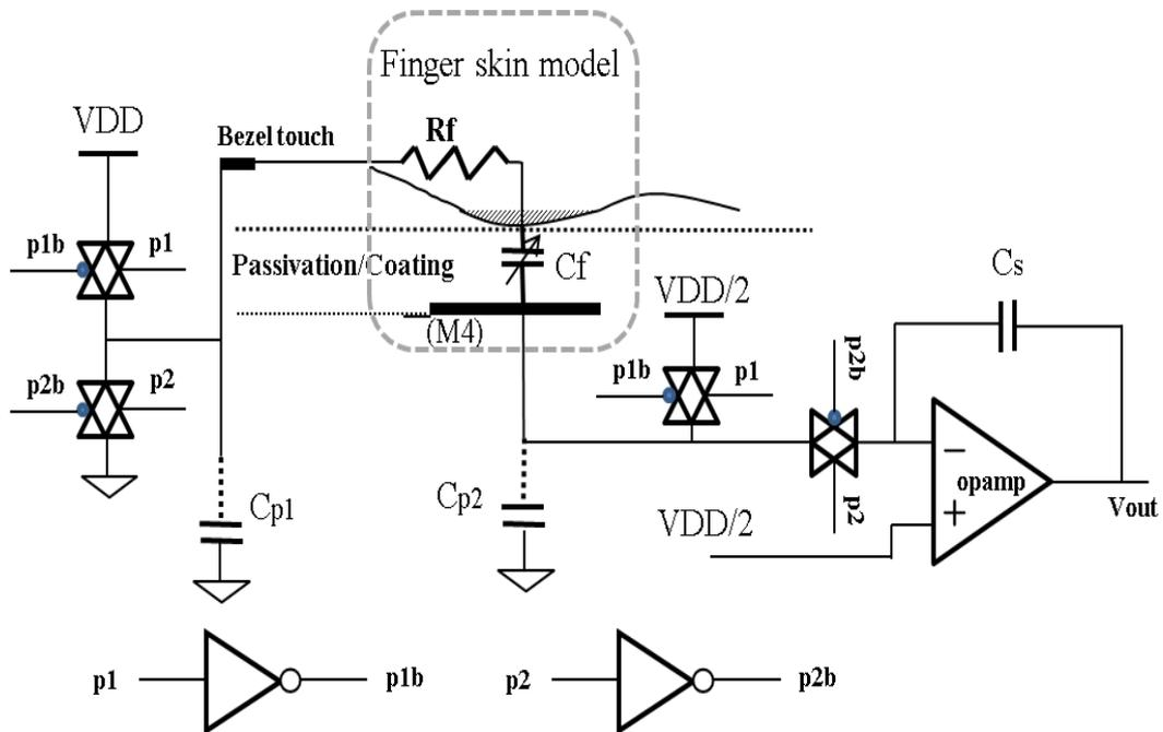
Figure 4. One Pixel Circuit of Proposed Sensor
