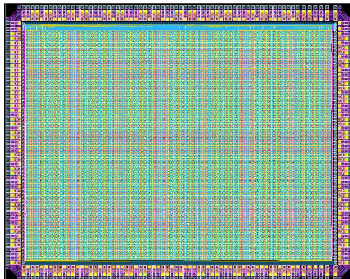
**Figure 10. 128x100 Pixel Array Chip Layout (8721  $\mu\text{m}$  x 6921  $\mu\text{m}$  @0.35 $\mu\text{m}$  CMOS Process)**
