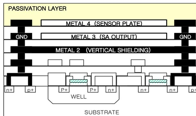
Figure 2. Horizontal and Vertical Isolation Structure of Typical Sensor
