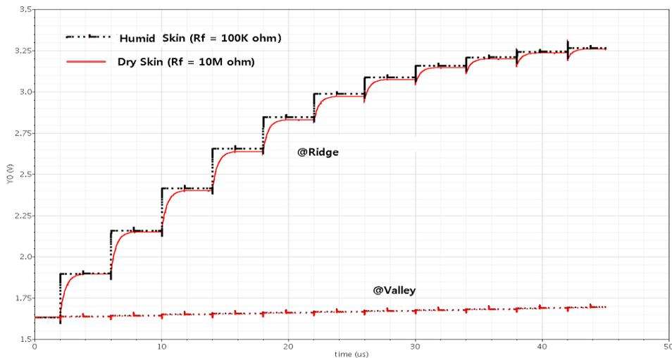
**Figure 7. Output Characteristics on Dry and Humid Skin (0.35 $\mu$ m Typical Parameter and 3.3V Power Supply)**
