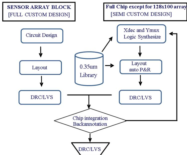
**Figure 9. Design Flow of Fingerprint LSI**
