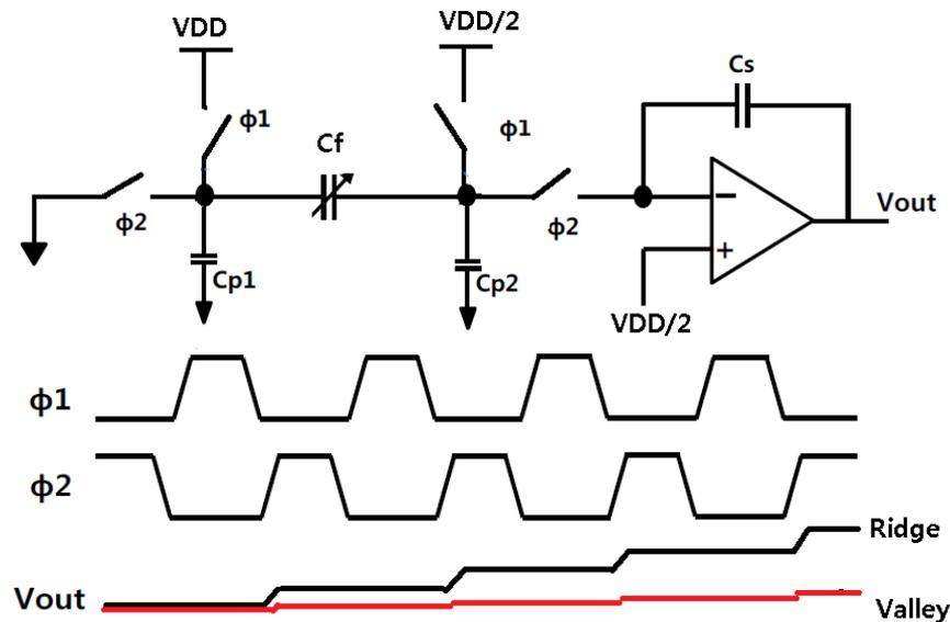
**Figure 3. Charge Transfer Switched Capacitor Integrator Circuit**
