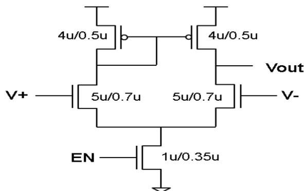
Figure 5. Simple Opamp for One Pixel Layout
