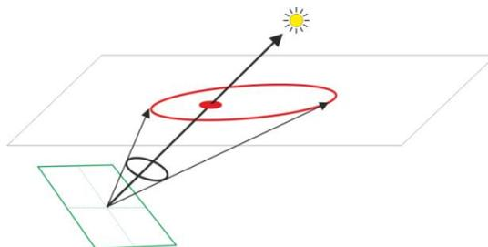
**Figure 6: Representation of the solution to (5) as a conic section (in this case an ellipse). The apex of the cone lies at the point on the surface, while its axis lies along the light source vector.**
