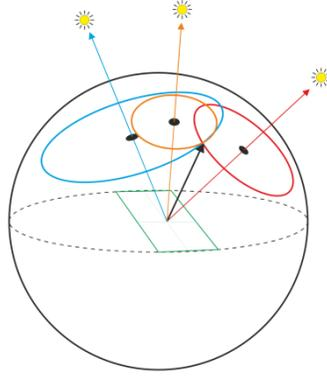
**Figure 7: Representing the solution to (5) on a sphere for three different light sources. Use of multiple sequential light sources are able to fully constrain the normal, as in PS.**
