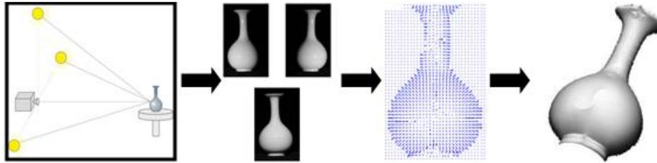
**Figure 1: Illustration of a basic photometric stereo capture mechanism. From left: experimental arrangement, raw images, estimated surface normals, recovered depth. The algorithm in [4] was used here to calculate depth from surface normals.**
