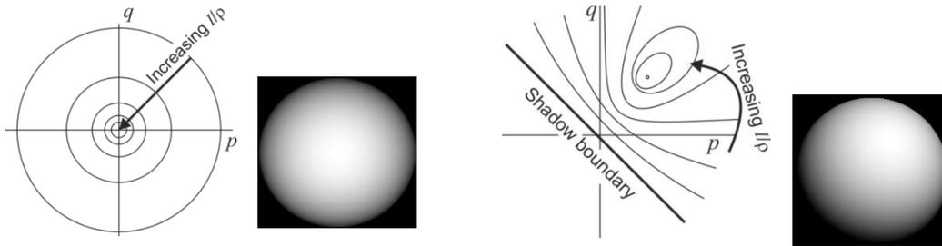
**Figure 5: Solutions to (5) for  $p$  and  $q$ . The left-hand example shows the case where  $p_s = q_s = 0$ , while for the right-hand case,  $p_s = q_s = 0.5$ . The rendered images show a Lambertian sphere illuminated under these particular light source directions.**
