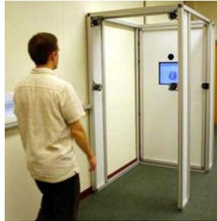
**Figure 8: A prototype PS face recognition device.**
