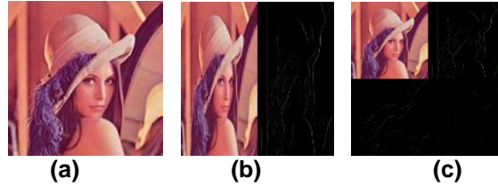
Figure 3. Non-standard Decomposition of an Image (a). Original image, (b). Decomposition of the row (c). Decomposition of the column
